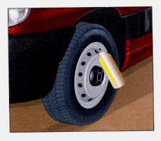
As your Electric Vehicle does not have a spare wheel, a temporary puncture repair aerosol can be found under the front passenger seat.
